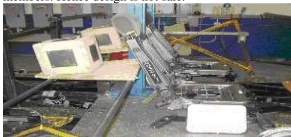
Figure 01: Sled Testing Set-up (Courtesy:- SAE Paper)
